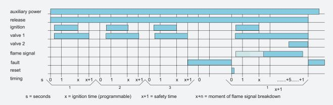
After failure and reset again all re-ignitions are available.
